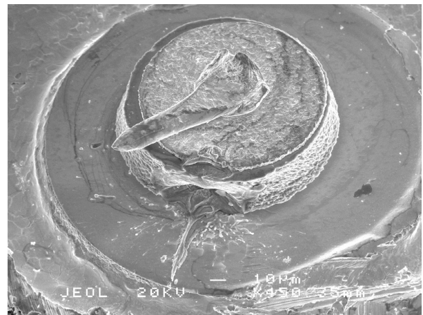
Figure 7.26 (above) SEM image of the EOS of a diode mesa
